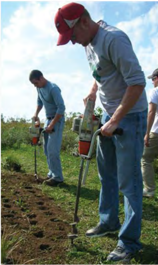
Figure 3-20: Power auger efficiently drills holes
