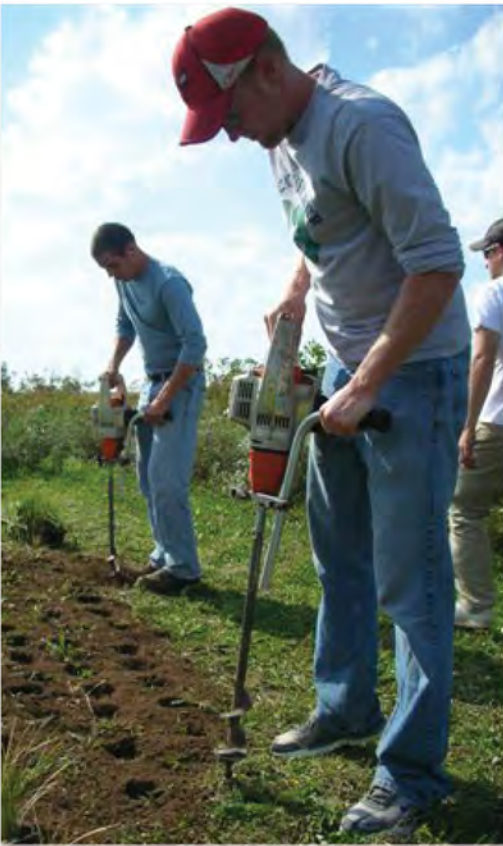
Figure 3-20: Power auger efficiently drills holes
