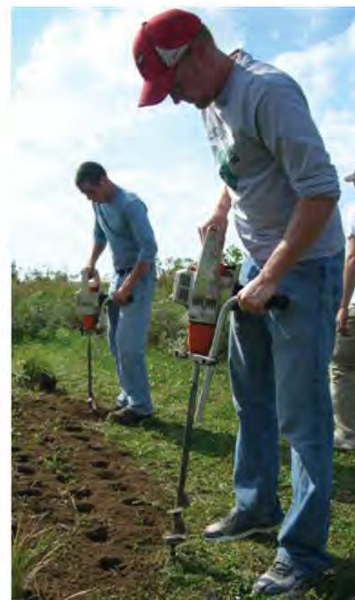
Figure 3-21: Power auger efficiently drills holes
