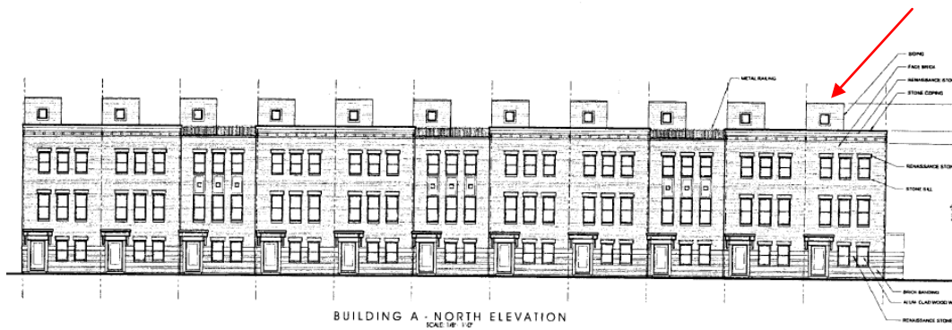
Figure 2 the arrow indicates the penthouse feature that is not incorporated on the proposed seven (7) unit building.
