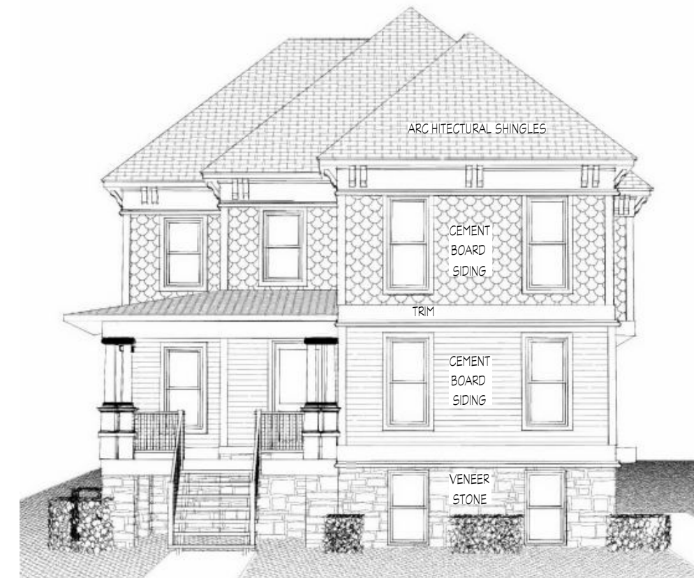
FRONT (NORTH) ELEVATION - ILLINOIS STREET
