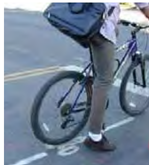
Bicycle detectors at traffic signals show cyclists where to place their bike for detection by demand actuated traffic signals.
